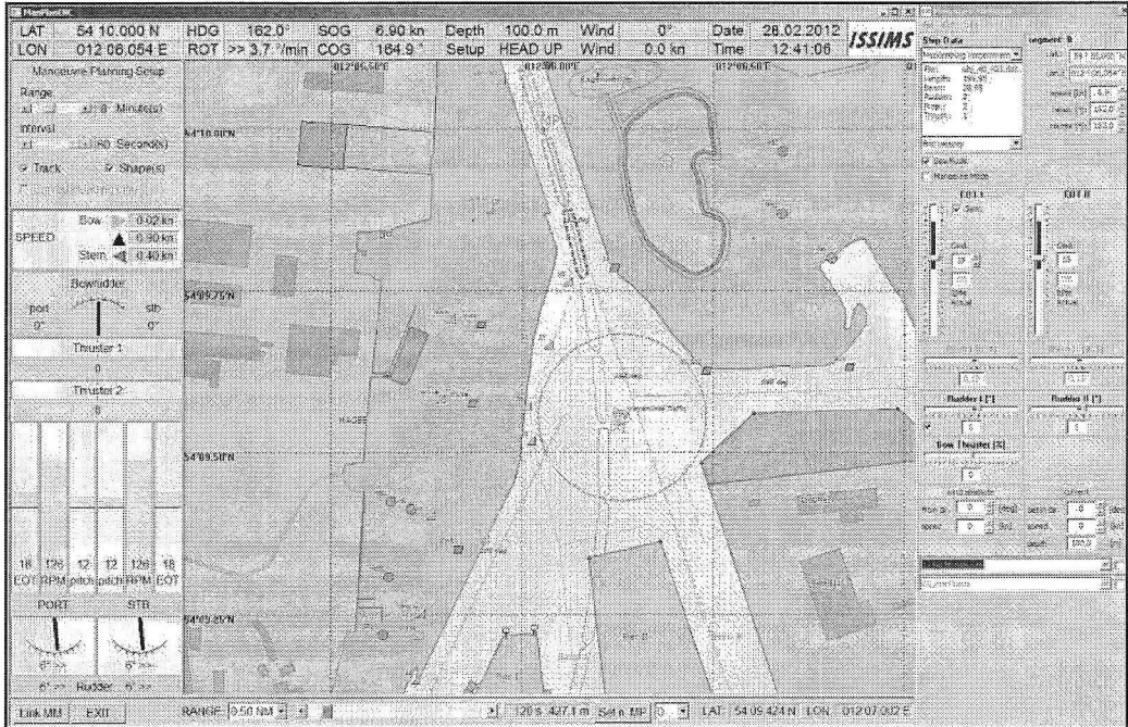
Figure 11 Display for Manoeuvring Design by Fast Time Simulation for immediate presentation of manoeuvring results: Sample for entering the turning area with slight turning to STB from initial conditions in a fairway at initial Manoeuvring Point MP 0
