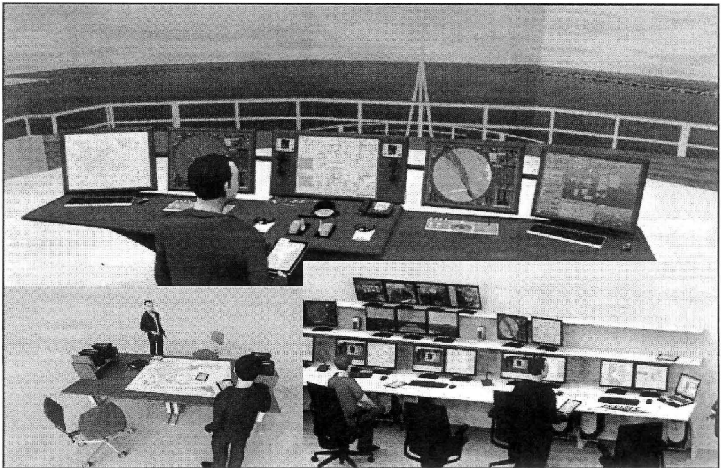
Figure 16 SAMMON System set up based on Tablet PCs within Ship Handling Simulator environment: as Bridge Version (top), Lecturer System (bottom left) and Instructor Version (bottom right)
